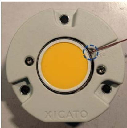
Figure 6: Typical T-type thermocouple attachment at the T<sub>C</sub> measurement location. Adhesive omitted for clarity.
