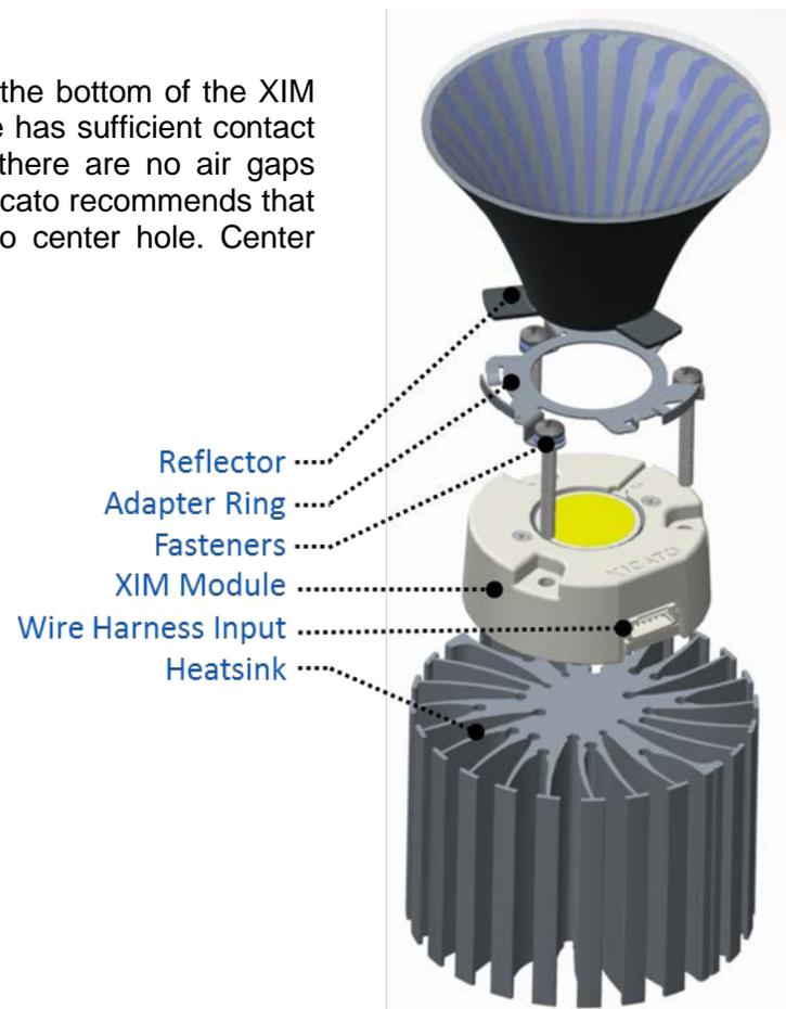
Figure 2: XIM Assembly (Exploded View)
