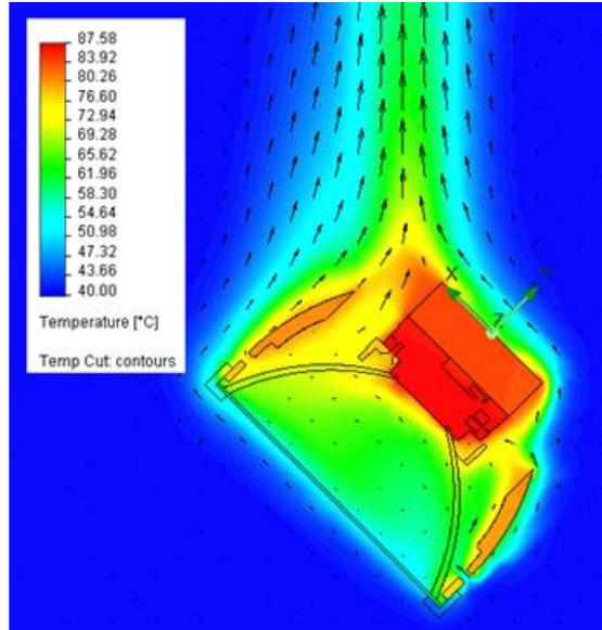
Figure 10 – Temperature distribution and velocity for example luminaire
