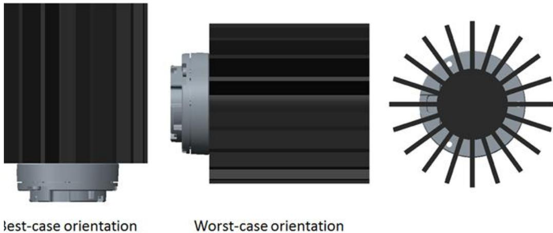
*Figure 2 – Preferred fin direction for 0° orientation*
