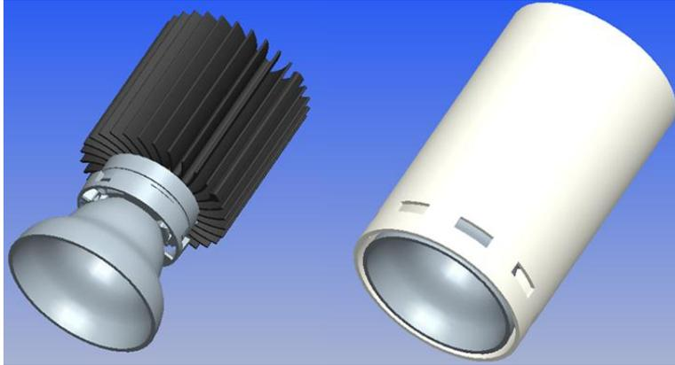
*Figure 13 – Module, heatsink, and reflector in free-air and inside a can*
