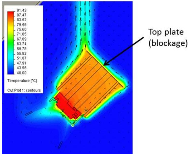
Figure 12 – Temperature distribution and velocity for Xicato HS w/ top covered
