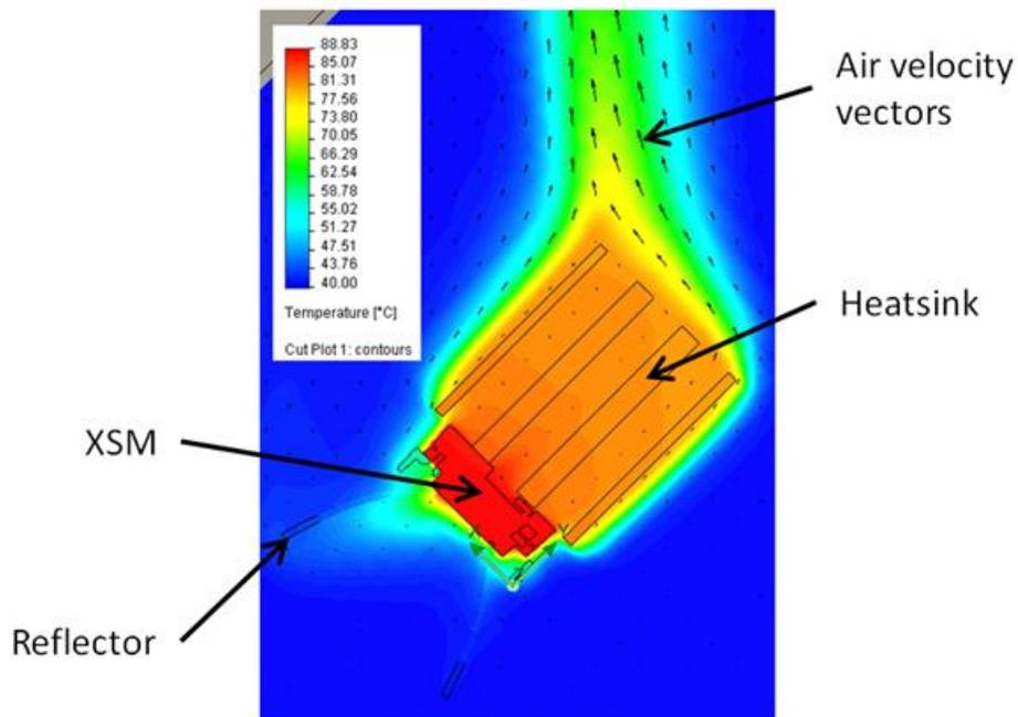
Figure 7 – Temperature distribution and air velocity for Xicato reference HS
