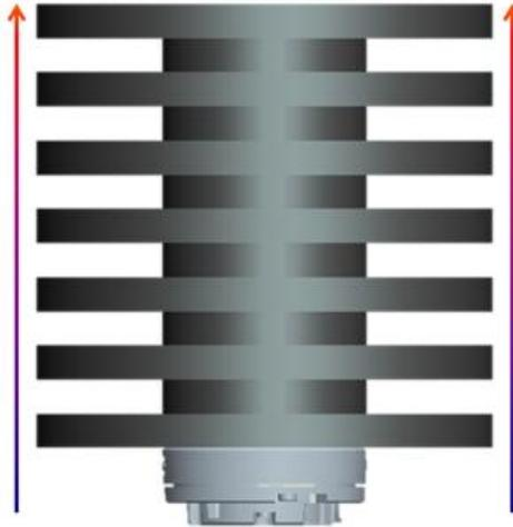
*Figure 3 – Poor fin design for 0° orientation*
