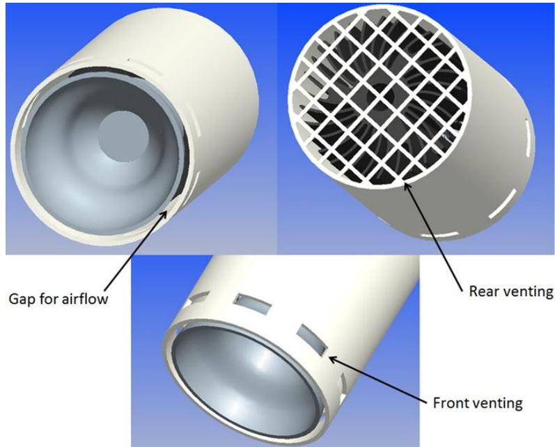
*Figure 14 – Possible venting options for an enclosed track spot luminaire*
