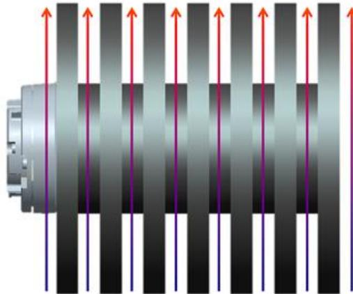
*Figure 4 – Good fin design for 90° orientation*
