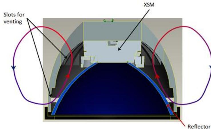
*Figure 9 – Airflow pattern for example luminaire*
