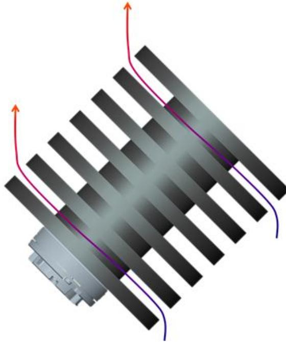
*Figure 5 – Possible good design for 45° orientation*
