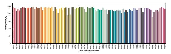
This chart displays the Fidelity Index for each of the 99 CES. The CES are arranged by their hue angle under the 5000 K reference source, which was also used to determine the color of each bar. The colors are approximate and depend on proper monitor calibration. Some colors may be outside of the gamut of the monitor, and will not be displayed accurately.
